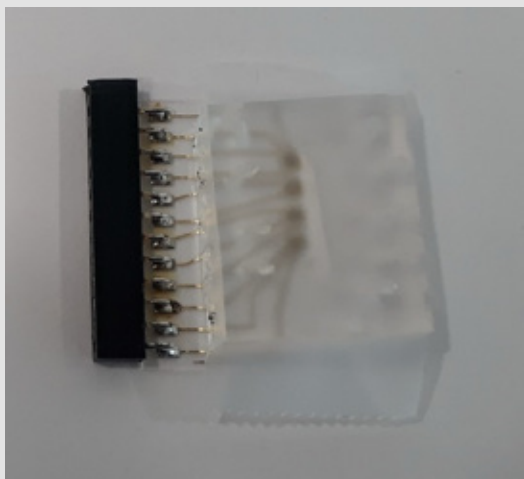
A pluggable microfluidic module for heavy metal ion sensing
